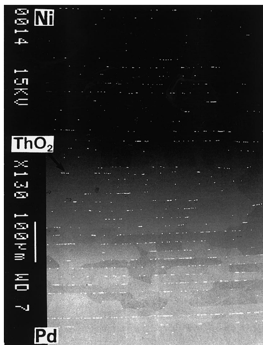
Fig. 9. Backscattered electron image of a Ni/Pd multi-foil diffusion couple annealed at 1100°C for 121 h in vacuum. The rows of \text{ThO}_2 particles used as fiducial markers correspond to the interfaces between the initial foils. Note: no pore formation after the heat treatment.
